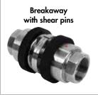
The shear pin Breakaway is designed to function with pull forces that are designed to pull at an angle of 10 degrees or greater from the center line of the Breakaway. The shear pins separate at a pre-designed force closing the valves. These type Breakaways are used on piping systems to connect hoses and loading arms as protection to prevent high forces that may break the loading arm or hose. It also protects the piping system from damaging pull forces.
